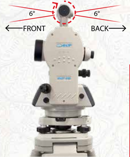
The laser diode rotates through 360° inside the Hexagon brass anodised housing - the beam exits front and back at a 6° arc, producing a pulsed vertical line.
